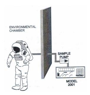
Suit pressures are below atmospheric pressure, so samples are drawn by vacuum pump to the instruments. Tests are performed to determine oxygen and moisture levels as the temperature inside the space suit changes.
